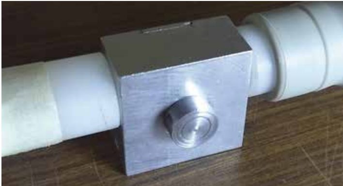
Figure 3: Paddle flow sensor connected to the Ventilator
